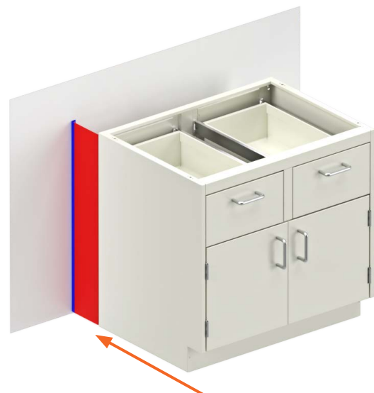
3 Use screws to attach the L-Filler to the base cabinet.
